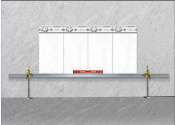
Aluminum bar supports the tiles during paneling process
